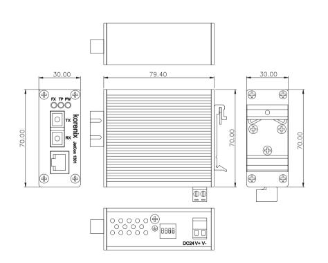
JetCon 1301 Industrial Fast Ethernet to Fiber Media Converter
